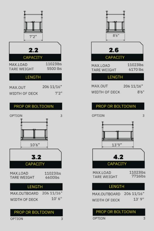
The world renowned Preston Rentals SuperDeck® retractable loading platform system has been designed to simplify the handling of materials, save hook time and rapidly improve productivity - particularly on multi-story construction sites. The SuperDeck's revolutionary design offers a 'drawer-like' loading platform system dramatically reducing crane loading times and delivering savings on labour costs - all while improving overall site safety.
